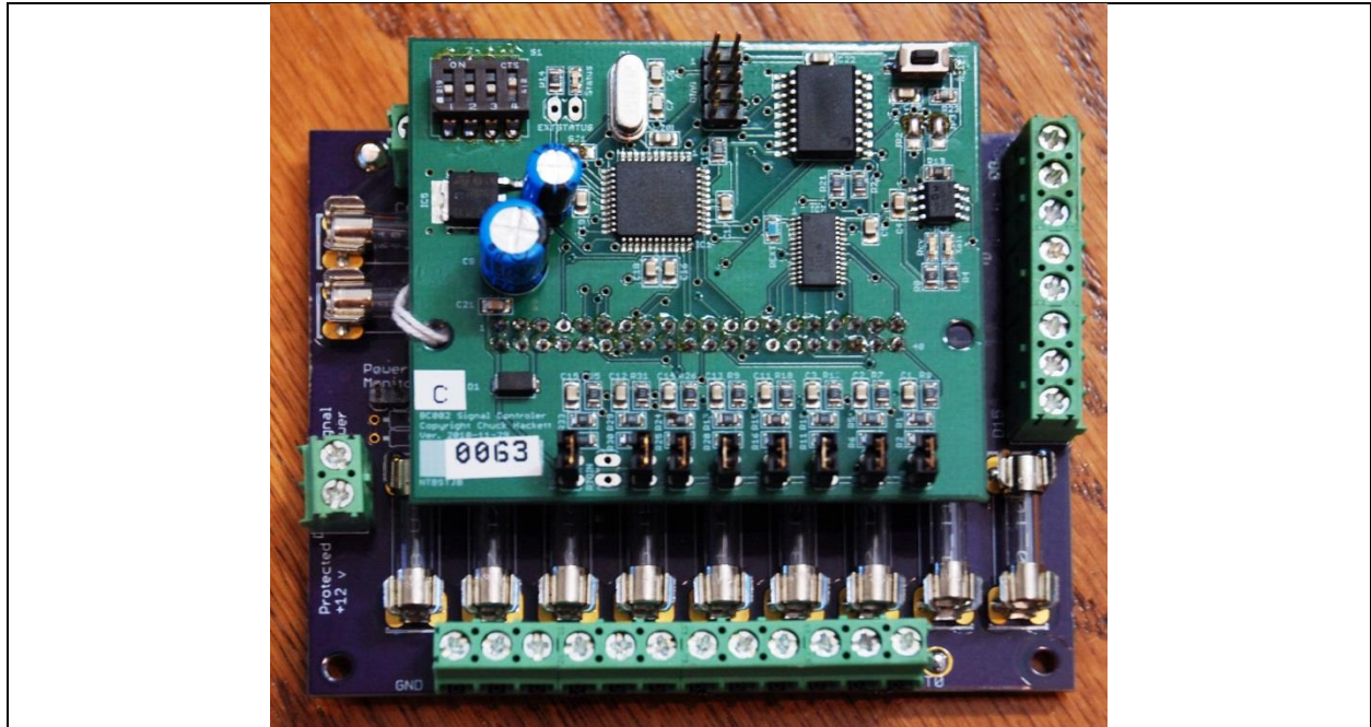
Base Board with controller installed
